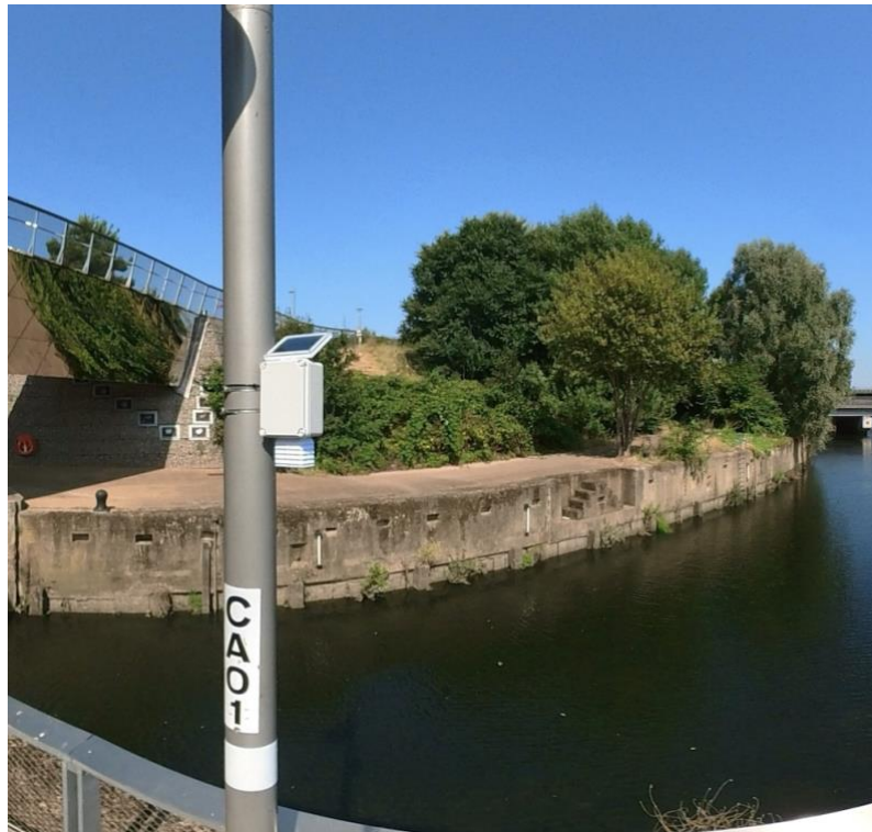
Figure 1 Solar-Powered IoT Sensor Deployed in QEOP for Microclimate Monitoring
