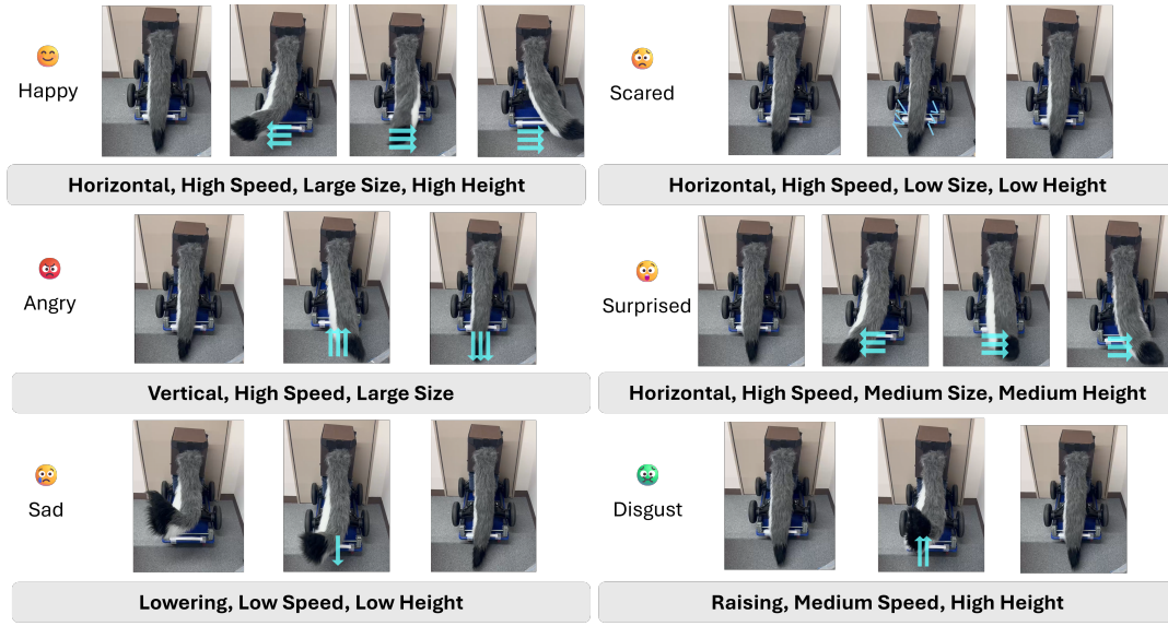
Figure 3: The tail motion we implemented to convey specific emotion by performing the designated sequence of motion parameters. The grey box shows the parameters, summarized in the mapping scheme, applied here.
