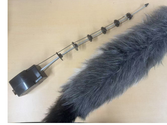
Figure 2: Implementation of our physical tail. continuum-type tail structure with 7 segments and fur.
