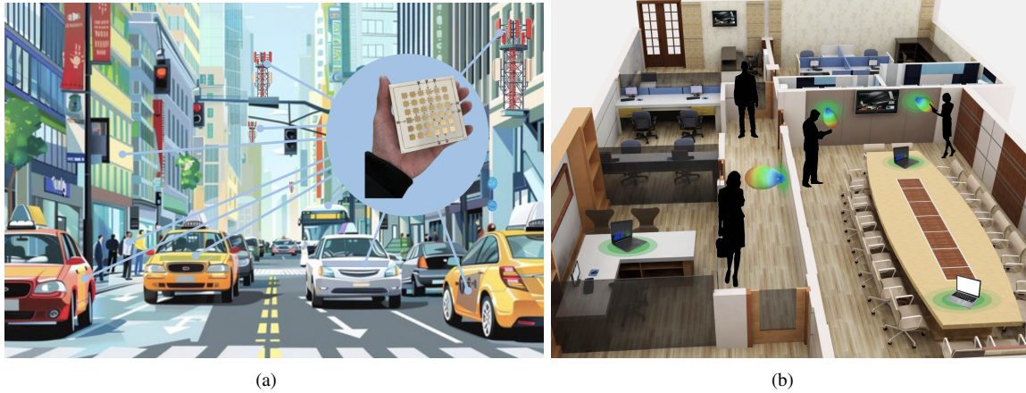
Fig. 1. Illustration of possible FAS deployments: (a) RPA-FAS used at base stations (BSs), user terminals, vehicles, and building surfaces, etc.; and (b) an E-FAS deployed in an indoor environment, where all reconfigurable surfaces collectively form a large FAS to serve users within the space. In this case, users are served via the shortest possible wireless links, and some may even be served through direct contact with the surfaces [7].
