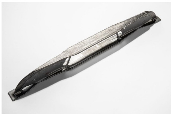
Fig. 14 The 3D printed MMTO beam following support removal and sandblasting (photo by Aaron Hargreaves/Foster + Partners)
