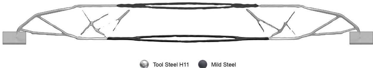
Fig. 2 The 10% volume fraction MMTO beam with a 60% mild steel and 40% tool steel distribution, showing the discontinuities in material distribution
