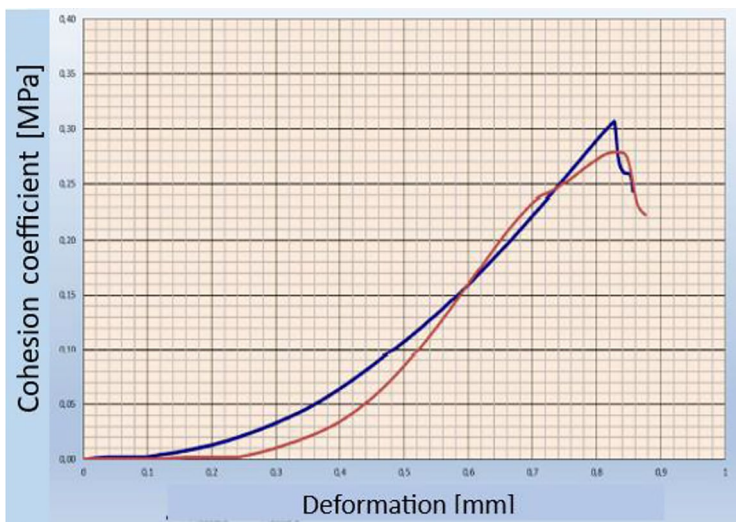
Fig. 21 Results of cohesion coefficient for samples B1 (blue) and B2 (orange)
