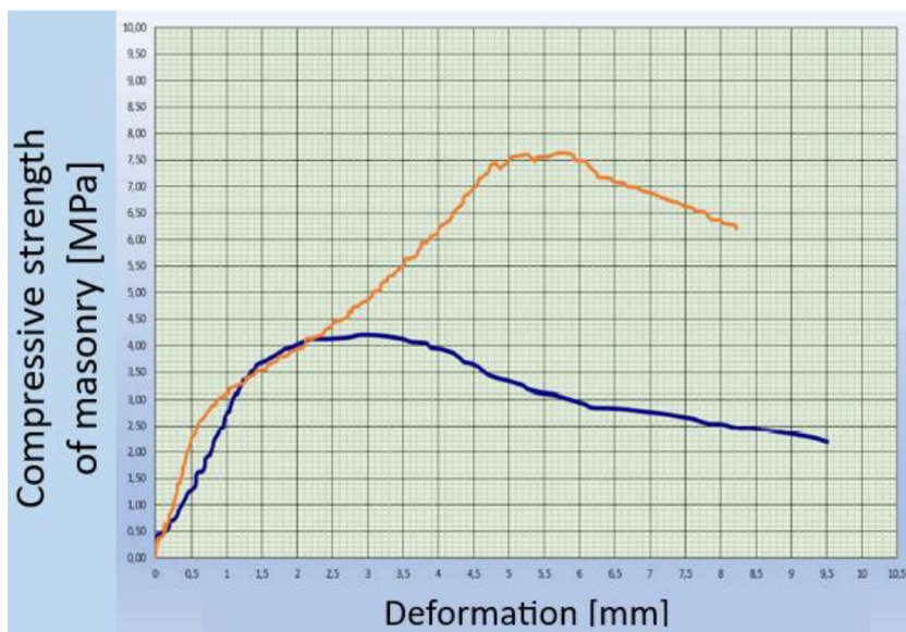
Fig. 19 Results of compression strength test of samples B1 (blue) and B2 (orange)
