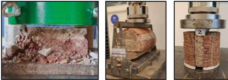
Fig. 17 Compression strength test (left), tensile strength test (center), and cohesion coefficient test (right)
