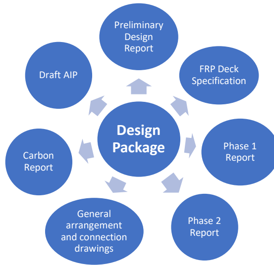
Figure 13: Components of the Design Package for the modular FRP-steel bridge.
