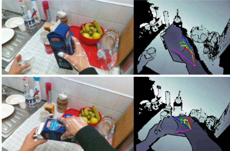
Figure 4.4: RGB-D video sample frames illustrating hand pose ground truth annotation using sensors. Left: RGB images with hand joint annotations, obtained via magnetic sensors strapped to the right hand. Right: Corresponding depth images showing the captured 3D hand pose. Figure adapted from Garcia-Hernando et al. [268]
