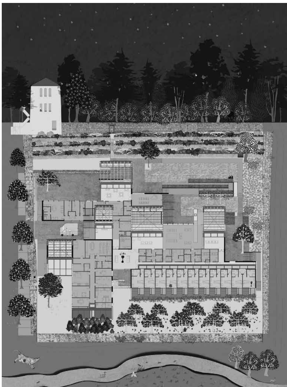
3 A 'daisy chain of high bright rooms looking onto gardens' and other dementia-friendly design principles, such as meandering paths that loop back on themselves, have been employed in the design of Níall McLaughlin Architects' Alzheimer's Respite Centre in Dublin, Ireland (2009).
