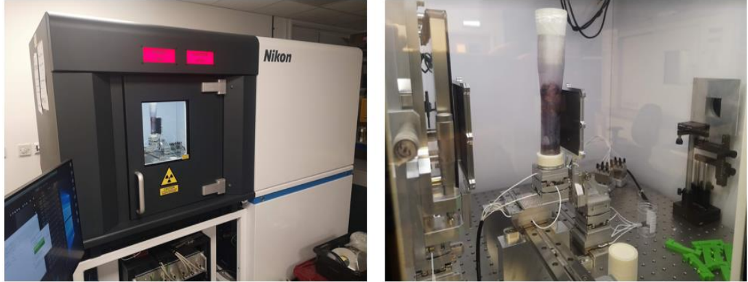
Figure 5.2: Images showing HICF machine. Left-hand image shows entire machine with radiation shielded enclosure. Right-hand image shows sample stage and masks.
