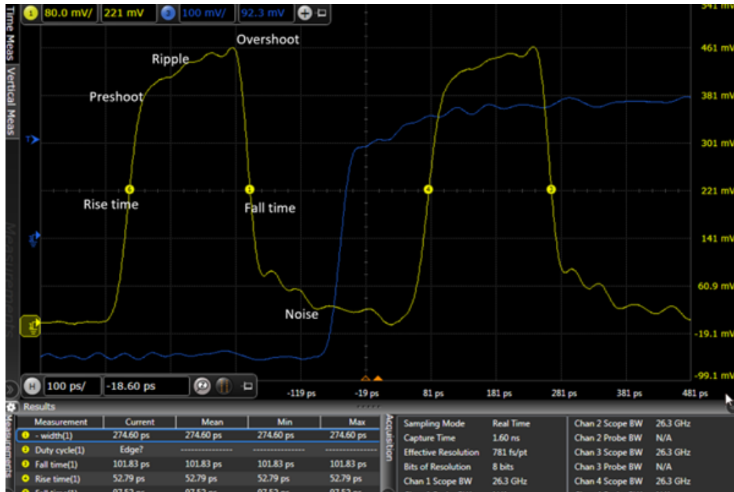
Figure 2.8: Pulsed measurement capture similar to Figure 2.7, except here the blue trace represents a marker output from the M8195A AWG that transitions high precisely when the second pulse is generated. In practice, this marker output is connected to a trigger input on the UHF instrument to indicate the onset of the second pulse, allowing a programmable delay to define the start of readout. In this example, the horizontal time axis shows the marker signal rising at approximately 19 ps, while the second pulse (yellow) returns to ground at about 281 ps, corresponding to a total delay of 300 ps between trigger onset and pulse termination. This delay value sets the timing offset for initiating integration or demodulation in the UHF system. Real-world waveform distortions observed in the first pulse (yellow) are annotated for reference.
