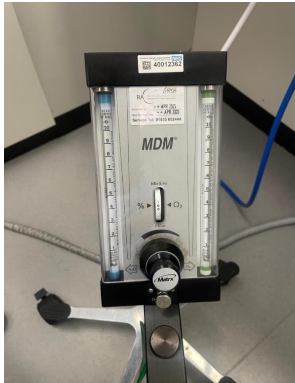
Figure 8: An example of a Monitored Dial Mixer (MDM) (Author's own)
