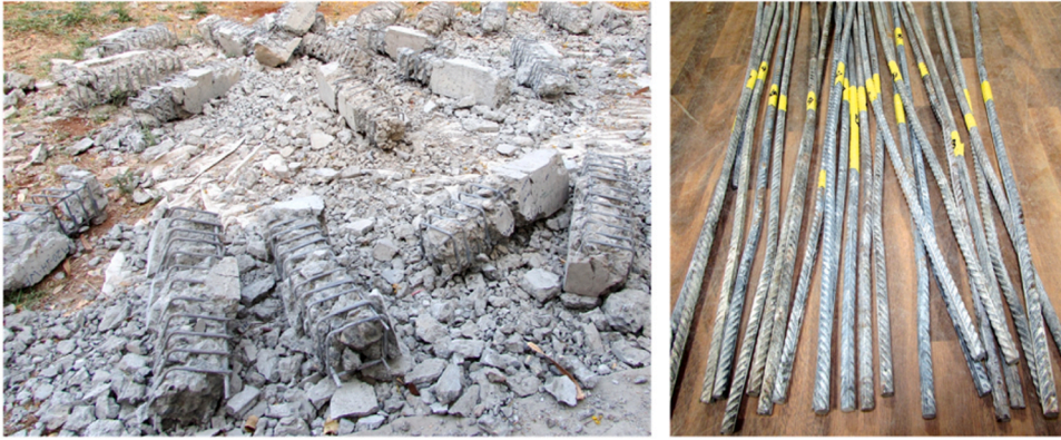
Fig. 24. Removal of reinforcing bars from test beams and the rebars employed for tensile testing.
