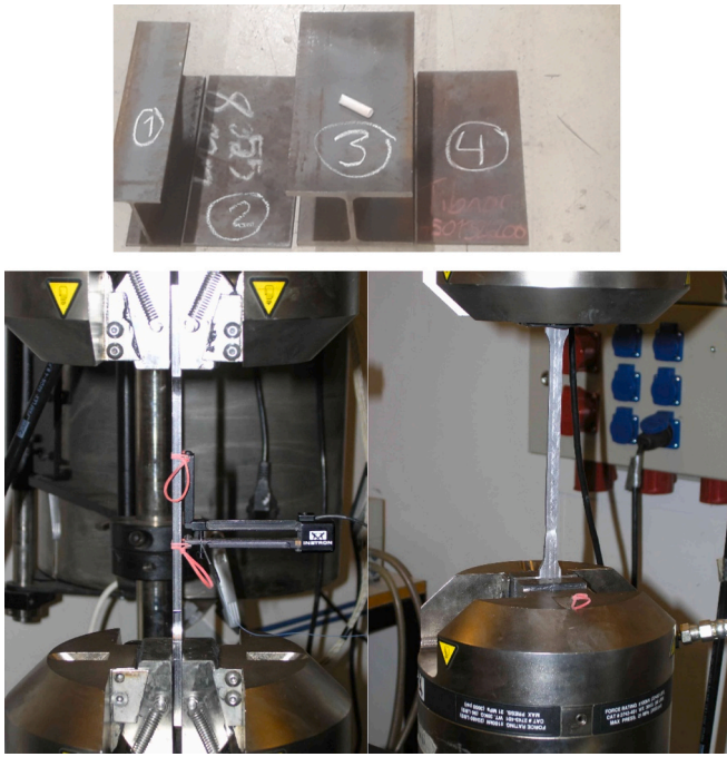
Fig. 5. Steel sections and plates from which the test coupons were cut for material testing.
