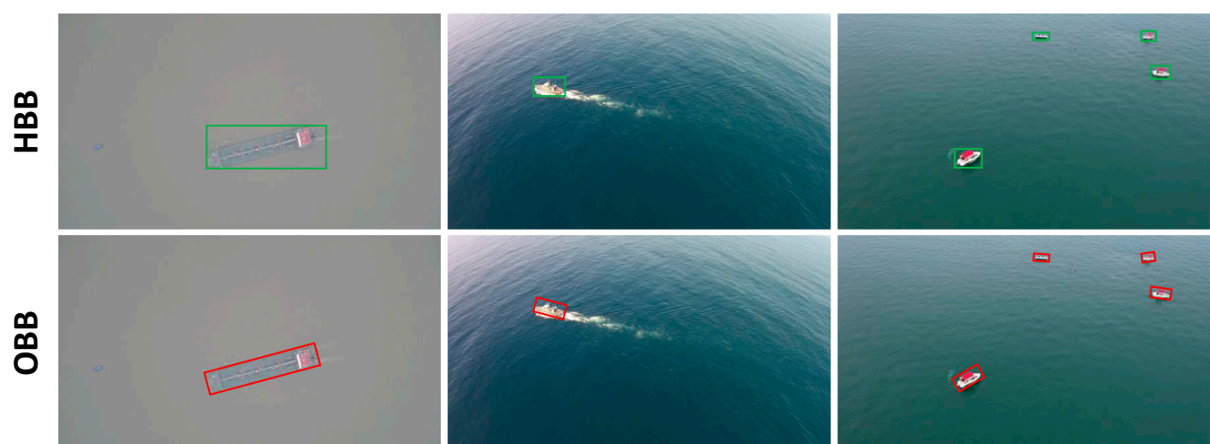
Fig. 2. Comparison of annotation methods between horizontal and oriented bounding boxes. The first row is annotated with horizontal bounding boxes, while the second row is tightly annotated with oriented bounding boxes.
