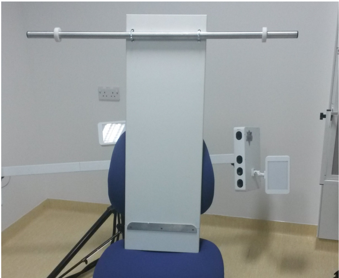
Figure 2.5. Image demonstrating the bespoke board designed and manufactured to keep the participant upright and arm position static above their head
