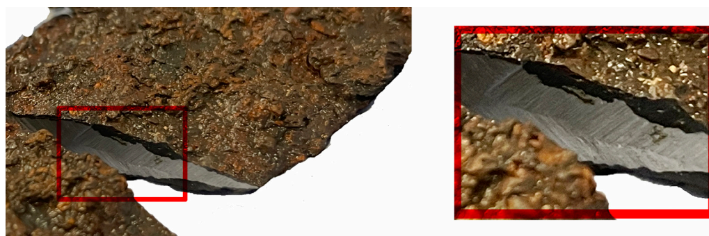
Figure 4 The spear after preliminary cleaning and sampling showing revelation of corrosion stratigraphy and metallic structure. Adapted from image provided by Fanxuan Fu
