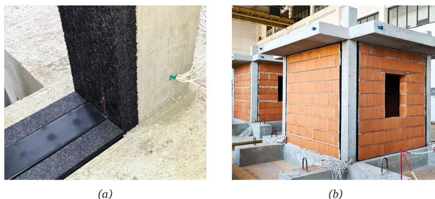
Fig. 4 Model 2 rubber joints. (a) Type 2 rubber joints placement. (b) Completely built Model 2.
