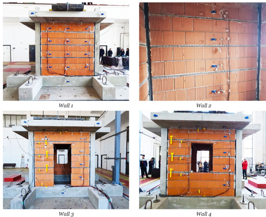
Fig. 15 Model 1. Instrumentation setup – Phase 2 – photos.
