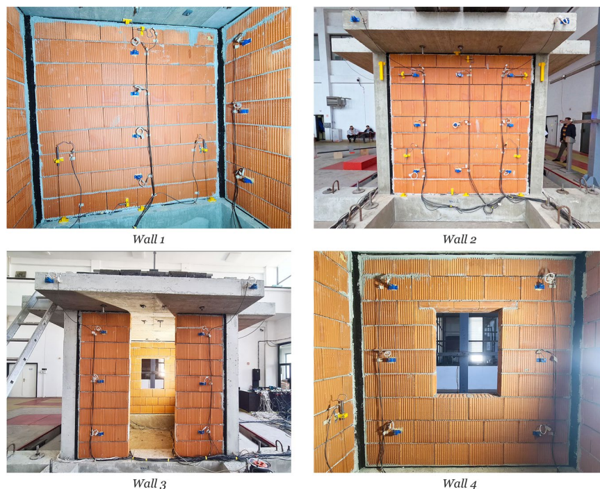
Fig. 21 Model 2. Instrumentation setup – Phase 1.
