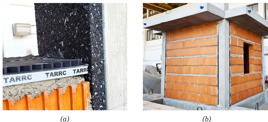
Fig. 3 Model 1 rubber joints. (a) Type 1 rubber joints placement. (b) Completely built Model 1.
