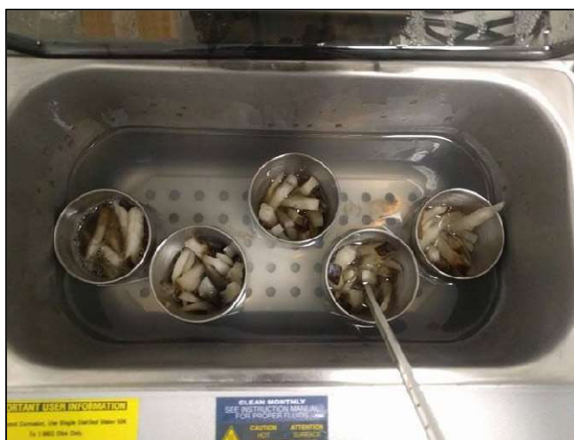
Figure 2.3: Image of initial diffuser model. Diffuser model consists of five stainless steel cups filled with cossettes. The cups are placed in a pre-heated water bath at the selected temperature. Buffer is then added to each cup in a stepwise process to maintain a counter-current gradient and mimic industrial extraction.
