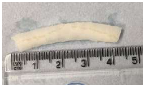
Figure 2.2: Average cossette dimensions and structure when prepared with the method used in this work. Dimensions of cossette are between 40-50 mm long, 2 mm deep and 6 mm wide.
