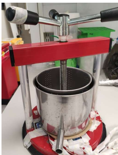
Figure 2.5: Manual press used in this study. The press is modified to ensure consistent pressure is achieved between replicates by use of a cable tie to prevent excessive screwing. A pressure sensor was also constructed by modifying 4 x 50 kg load cells connected to an Arduino Uno with an accompanying HX711 amplifier.
