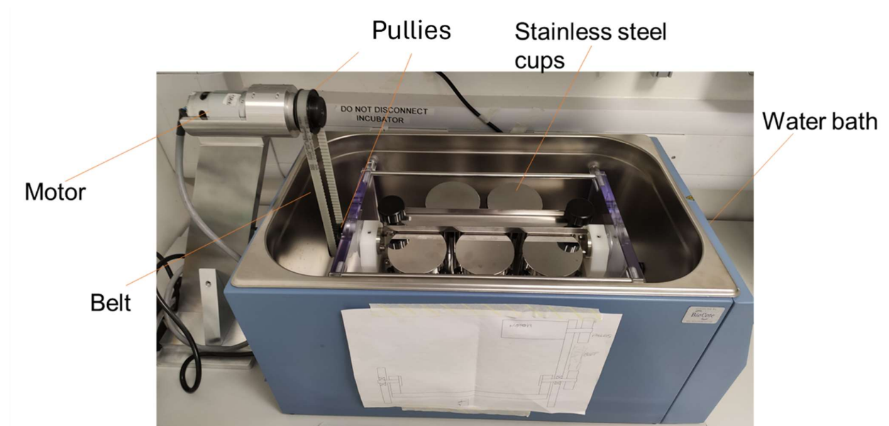
Figure 2.4: Image of the final diffuser model. A power generator enables the motor to rotate, causing the attached pullies to rotate. The pulley on the motor is connected to a pulley on the diffusion cup module via a belt, resulting in rotation of the diffusion cups as the motor rotates. This equipment was constructed in collaboration with the High Precision Design and Fabrication Facility (UCL Department of Biochemical Engineering).
