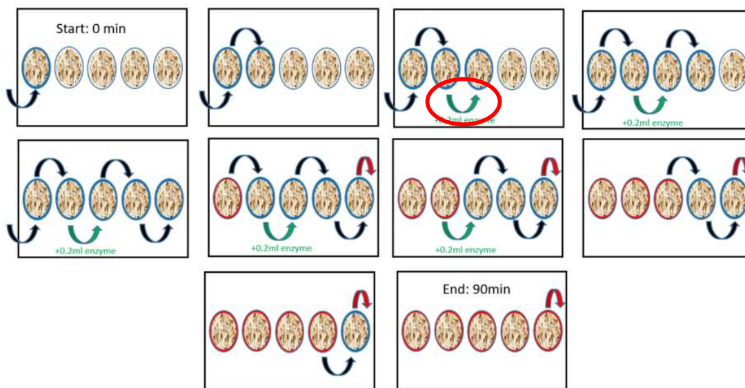
Figure 4.17: Water midpoint enzyme addition in counter-current diffuser model. Enzyme is dosed at the point where the water is midway saturated as it has been exposed to two cups of cosettes.
