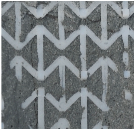
Fig. 20. Internal cracks of U-HPC at a strain rate of around 50 s -1 .
