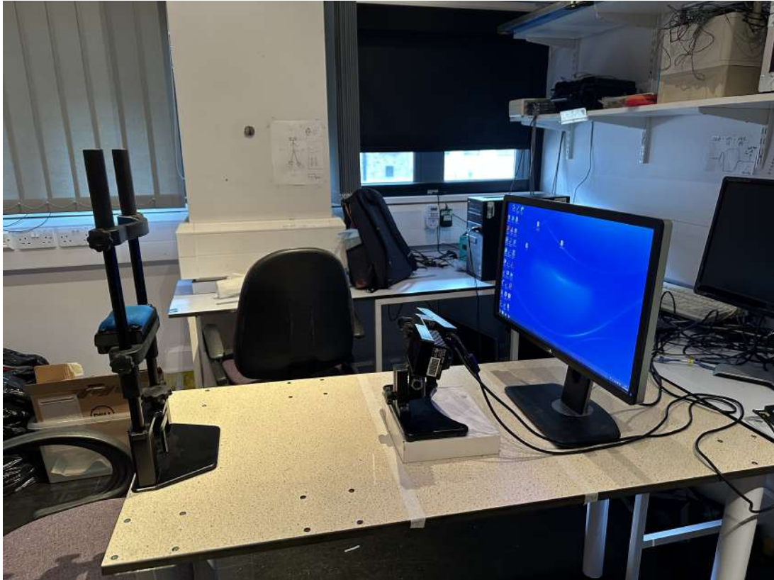
Figure 17: The EyeLink 1000 Plus in Head-stabilized Mode. The system comprises a host PC for participant setup, real-time detection and a display PC for stimulus presentation and data storage. Figure by author.
