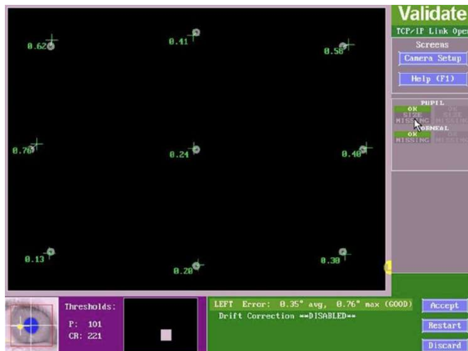
Figure 23: Validation Screen from the EyeLink 1000 Plus System. Recorded gaze positions and error values; the system calculates the average and maximum error, ensuring calibration accuracy before proceeding with data collection. Figure by author.
