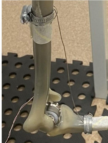
Figure 6-5: Assembled elbow implant with the humeral and ulnar stems joined together via posterior locking screws.
