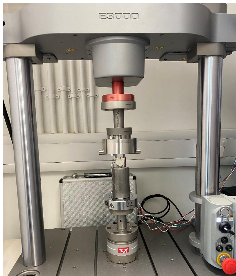
Figure A -1-1: Illustration of fatigue test setup for the strain gauged sample using the E3000 Instron machine.
