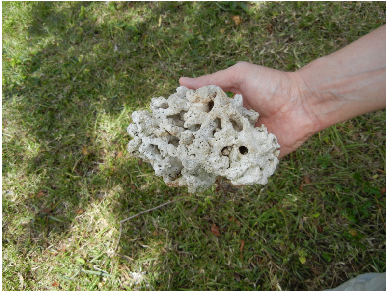
Figure 5.1 A piece of coral used for building, from the site of Jumba la Mtwana, Kenya. Source: author.
