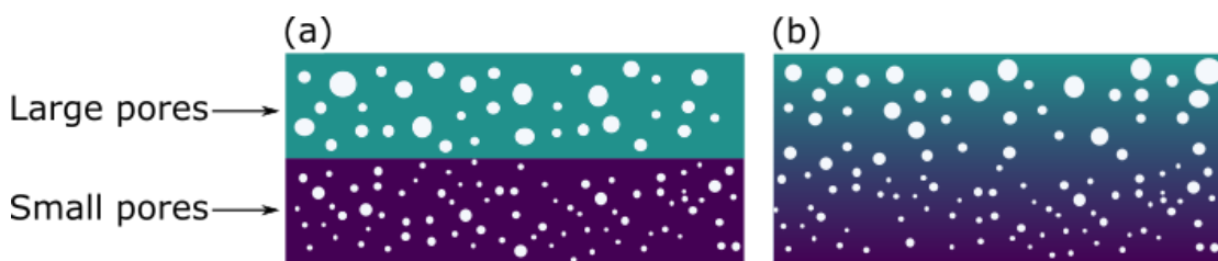
Figure 2-9: Illustration of a bilayer (a) and gradient (b) structure of two different porosity materials.
