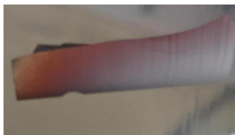
Figure 5-7: The colour change of LLZO coated LFP after 600 °C sintering. Red, LFP; White, LLZO.
