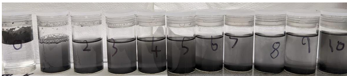
Figure 4-4: Dispersion test of 1 \text{ mg mL}^{-1} carbon black in different ratios of water and IPA. Each number on the vials represents a 10 wt% increase in IPA.
