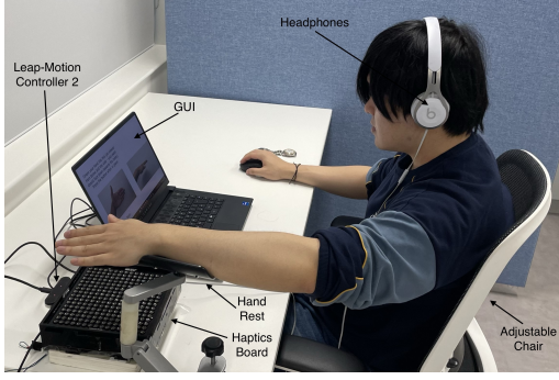
Figure 4: The set-up for the user study. The user sit on an adjustable chair and were provided with an arm rest to position the hand comfortably above the haptics board. The Leap-motion controller 2 tracks the hand and a python-based GUI allows the user to interact with the study. While the user is conducting the study, pink noise is played to avoid any device noise impacting them.
