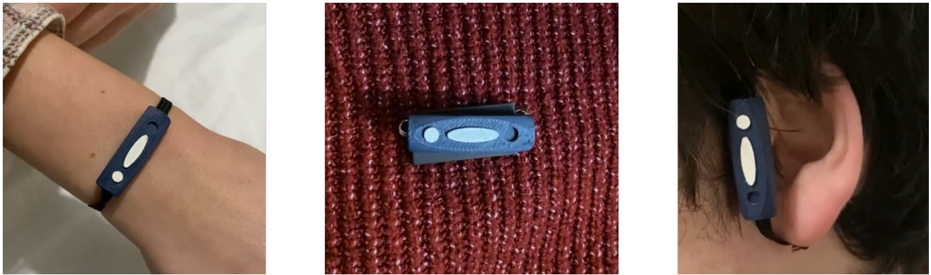
Figure 2: Iterated prototypes made of wire and paper, clay, and 3D printed materials in the left, middle and right image, respectively
