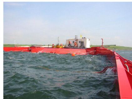
(b) Wave Dragon prototype in operation. Extracted from [11].
