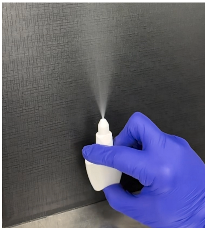
Fig. 7. Atomisation of engineered emulsions stabilised with 10 wt% BCS through unit dose nasal device (NasaDose) (Recipharm, 2023).
