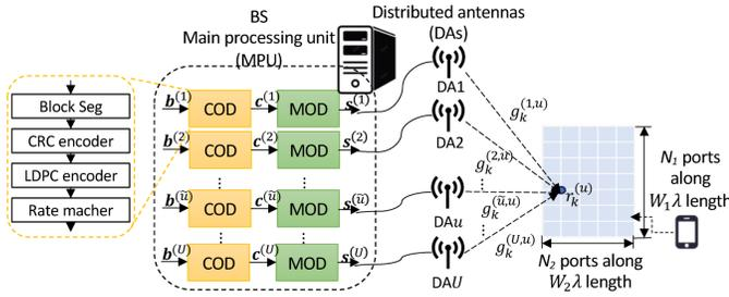
Fig. 1. System model of the coded FAMA system to a particular UT.
