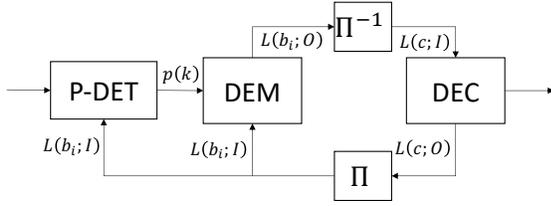
Fig. 2. The proposed iterative decoding receiver in the coded FAMA system.
