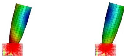
(a) Projectile entry at time  $t$  (b) Projectile at time  $t + 3.6 \times 10^{-3}$  s
