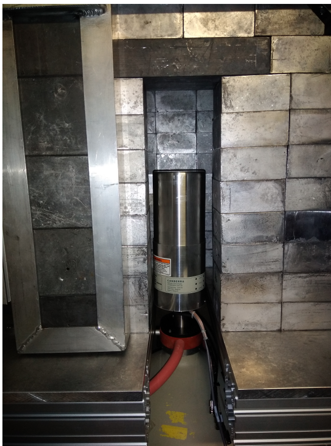
Figure 6.1: Photo of the HADES setup with the vacuum cryostat in the centre surrounded by the lead castle.
