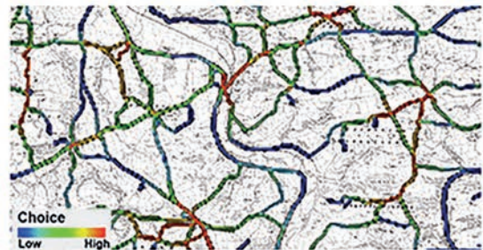
(c) Choice radius 2km - Space Syntax Open Mapping, overlaid on 1900 Ordnance Survey
