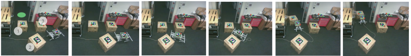
Fig. 7. Left to right: [t=0] Green dot is the goal. The robot: [t=4] avoids collision with object 3; [t=8] moves box 2 to create small opening; [t=10] stops pushing object 2 and rotates towards box 1; [t=12] pushes object 1 out of the door. [t=23] Goal reached. The robot performs non-axis-aligned pushing.
