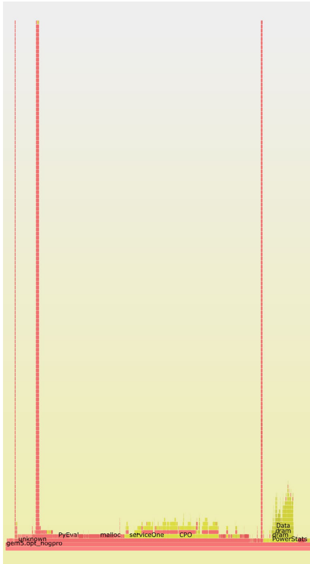
Fig. 2 FlameGraph of Linux perf profile of gem5 simulating our RNAfold fragment (Section 4.2). Used functions are spread horizontally, whilst vertical axis indicates depth of function call nesting. (An interactive version is available via https://github.com/wblangdon/Deep-Imperative-Mutations-have-Less-Impact )
