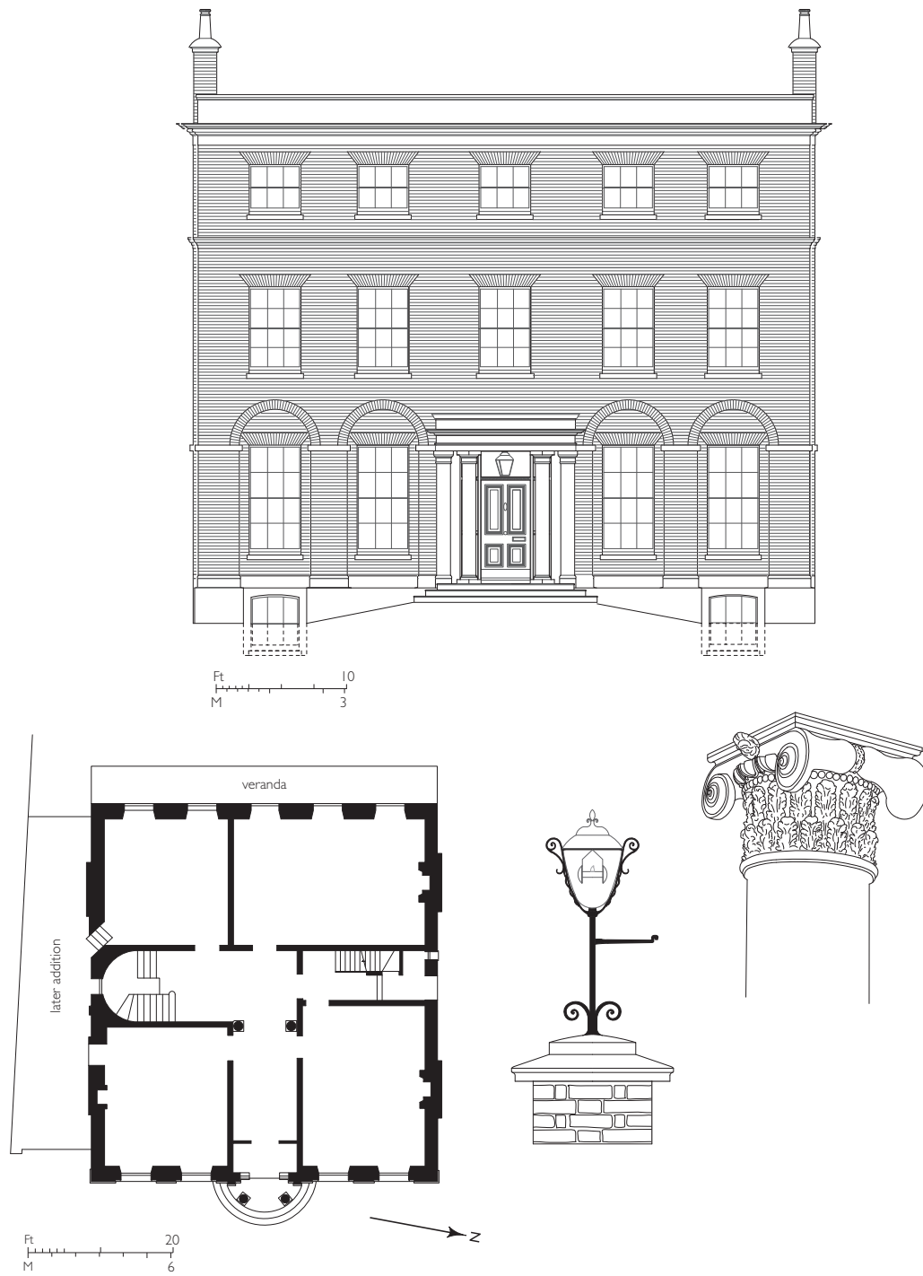
373. 21 Clapham Common West Side, elevation, ground-floor plan and details of cast-iron lantern on gate pier and column capital in entrance hall. Thomas Poynder, builder and developer, 1805–6
