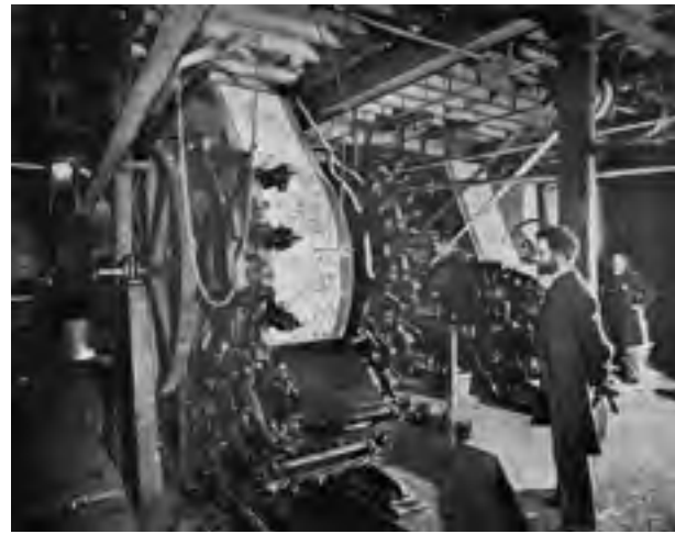
416. Printing wallpapers by machine at Essex & Company's paper mills, Lavender Hill, c.1899
