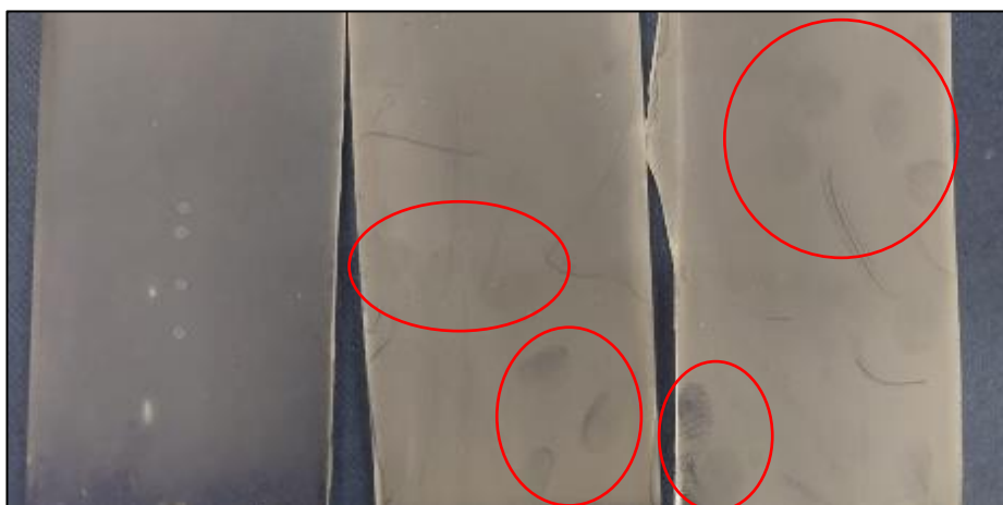
Figure 1.07. Photographs of a “well-adhered” film (far left) and “powdery” films (middle and far right). Finger marks are circled in red which can be seen in the “powdery” films.
