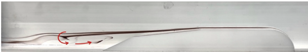
(c) Re-circulation is identified.
