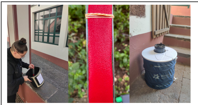
Fig. 2. Ovitrap (left image), a BG-Sentinel trap (right image) and red-paper with some stick eggs (middle image)
