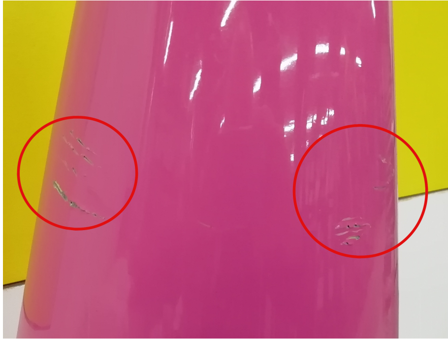
Figure 2.1: Shark bite marks on Seaglider operating in UK waters - courtesy of NOC.
