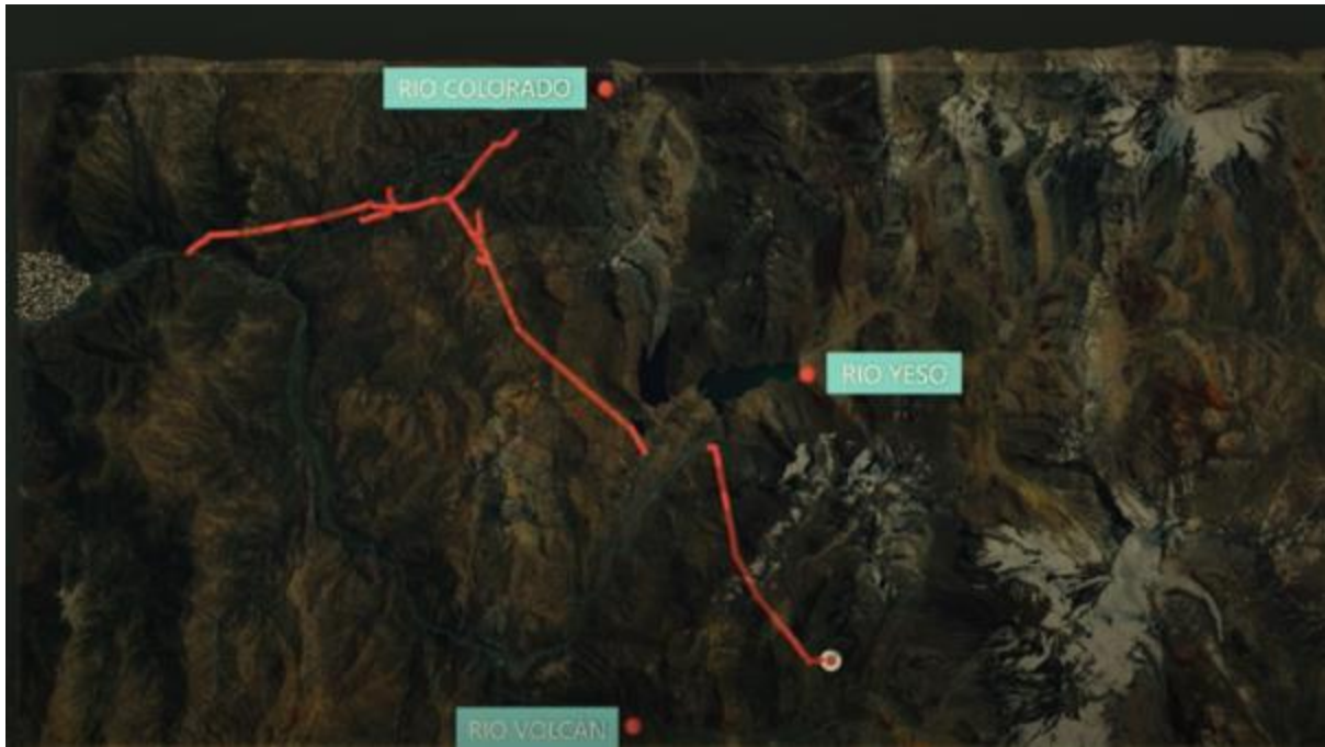
Figure 25. System of tunnels and the process of water collection from three different rivers: Río Colorado, Río Yeso and Río Volcán.(Source: Defiende Maipo)
