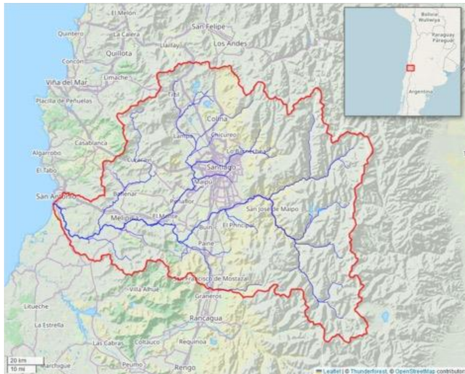
Figure 18. Analysing the tributaries of the Maipo River. Map and network of the Maipo River watershed. Created with the free Global Watersheds web app. Permalink to interactive map: https://mghydro.com/watersheds/shared/3ECB2F.html
