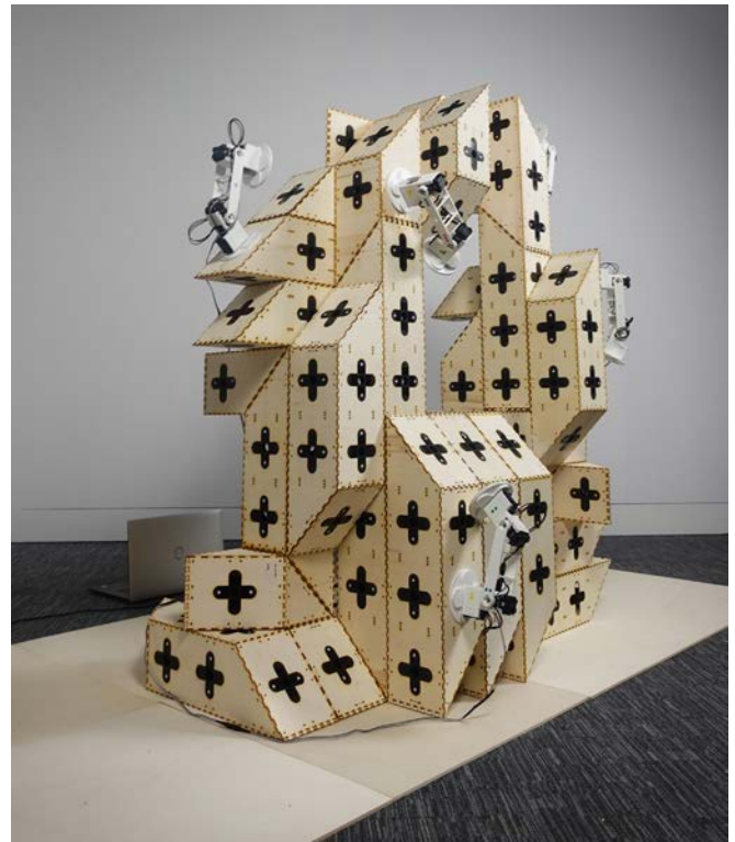
2 Photograph: Autonomous Collective Robotic Reconfiguration (ACRR), 2.4 m arch configuration.
