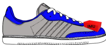
Figure 3. Placement of an IMU on top of right shoes above the toes.
