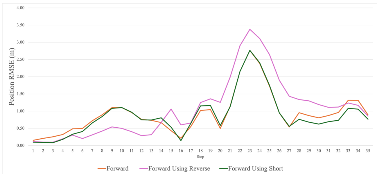
FIGURE 3 Forward Path posterity SLAM horizontal error per step
