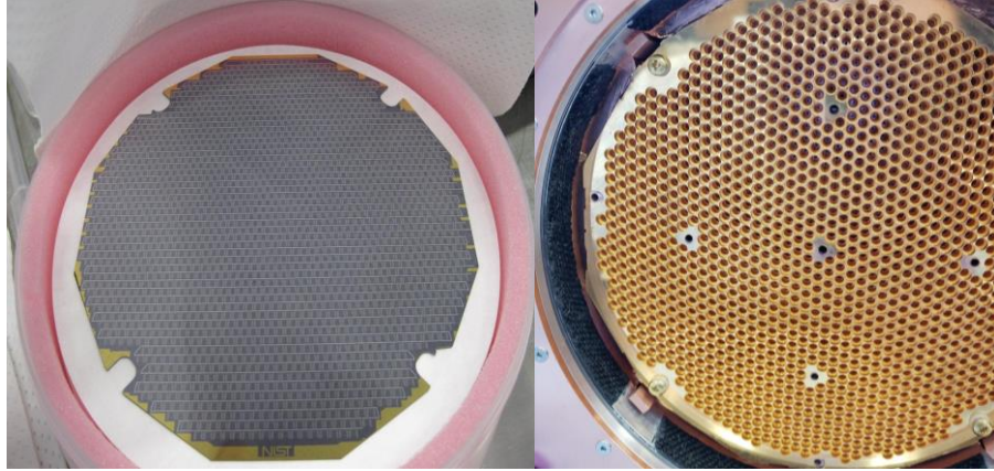
Figure 1. The detector array and feed horn structure fabricated by NIST for TolTEC [7] . It will consist of 3636 pixels at 1f\lambda spacing intervals, with 2 MKIDs detectors orthogonally polarized for each pixel. The incidental light will be feed horn coupled, reducing the stray light which has been a problem for SCUBA-2.
