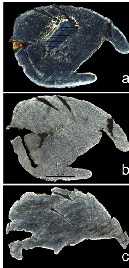
Figure 7. Silver inlaid: (7a) before cleaning with extensive C tarnishing (hatched surface), (7b) after cleaning with BR, (7c) after cleaning with WP
