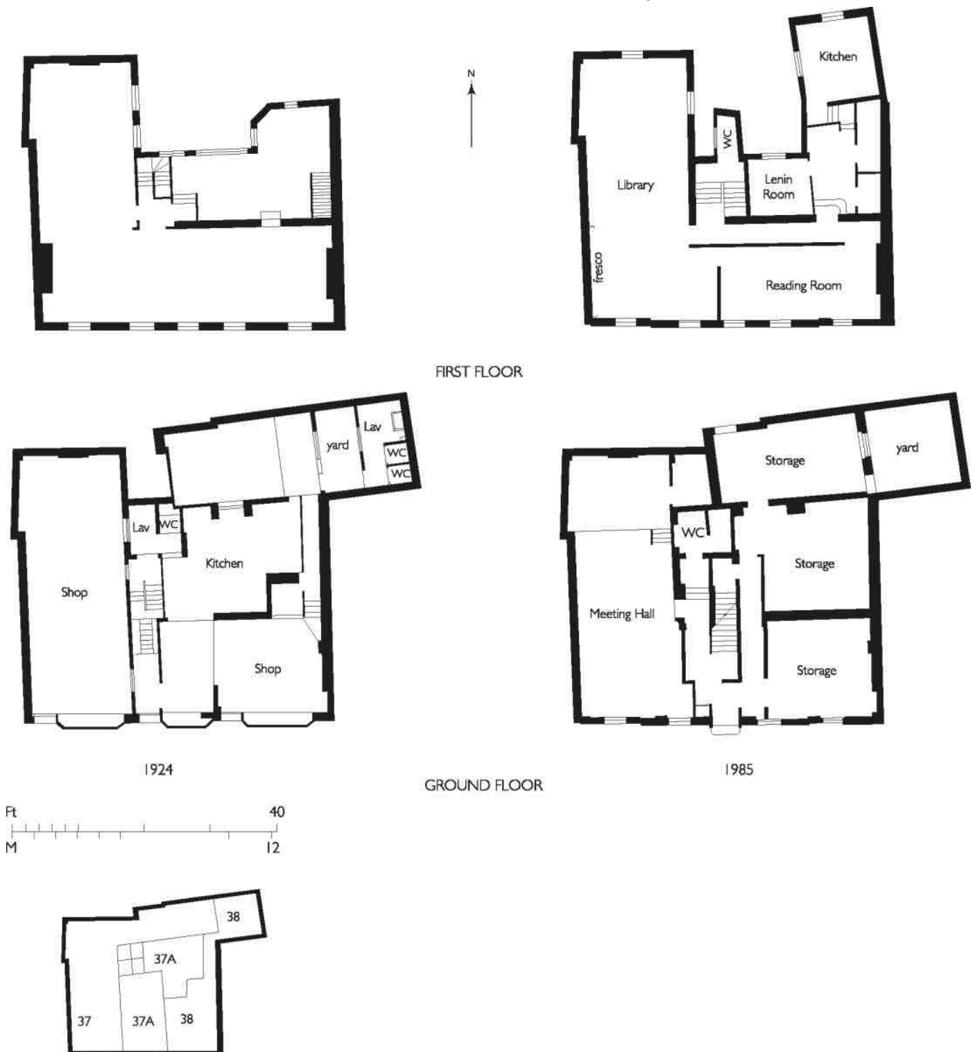
122. No. 37A Clerkenwell Green. Ground- and first-floor plans in 1924 and 1985, and block plan in 1884
