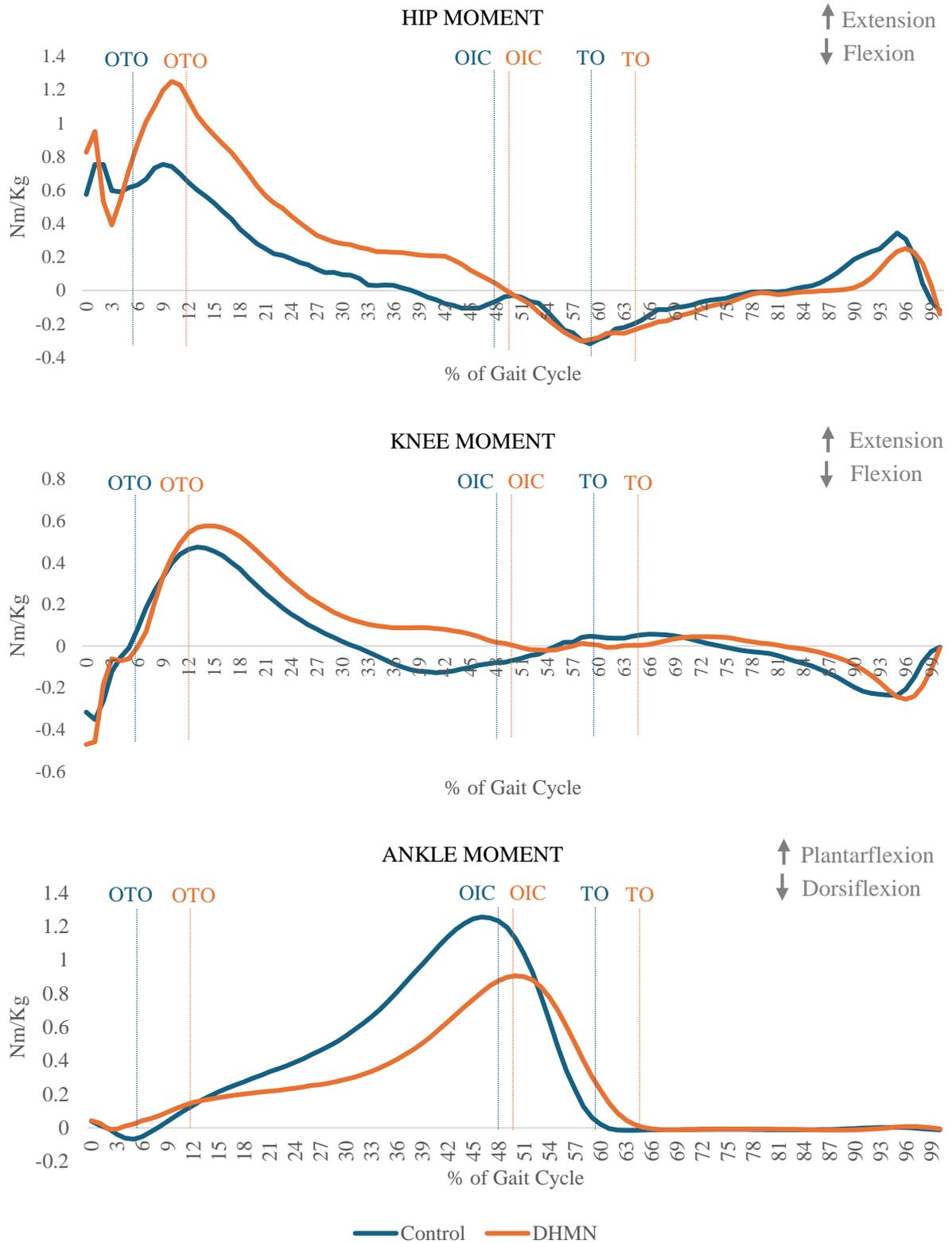
Figure 16: Grand average joint moments in the sagittal plane over one gait cycle for the ankle, knee and hip (average of left and right sides).
