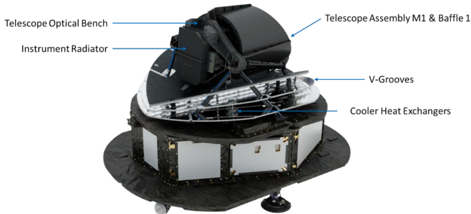
Figure 2-2: Illustration of the rear of the Ariel PLM
