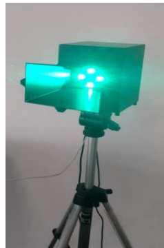
Figure 1. MSI imaging device used in the present work. The CMOS monochrome camera is positioned at the center, meanwhile the LEDs are mounted around it. The LEDs are covered by polarizing film to exclude specular reflection from the diffuse reflectance images.
