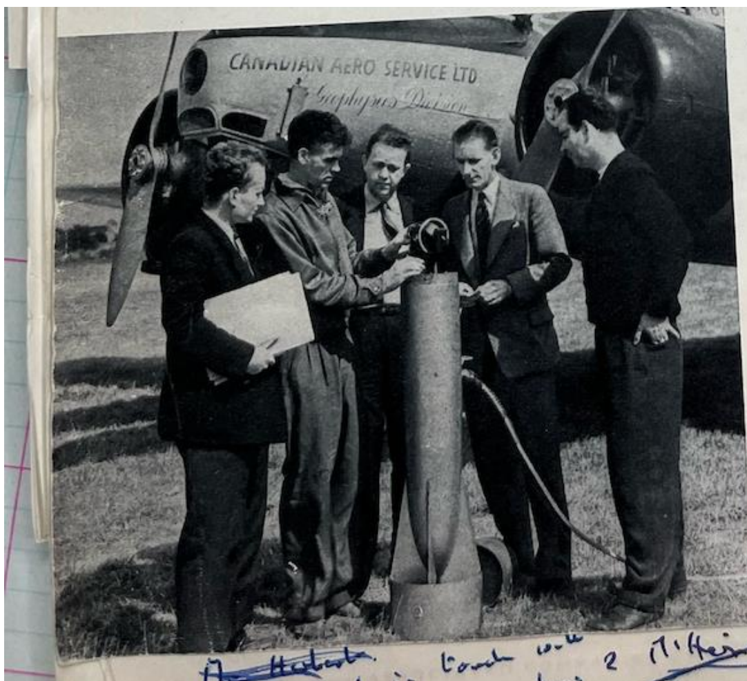
Figure 6.3. The “Tornado-shaped ‘Bird’” where the detector head was fitted, as mentioned in the Flight magazine report. From: ‘Midlands Survey - by
